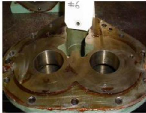
Rear cylinder plate Varnish: 9.6 Sludge: 9.6
