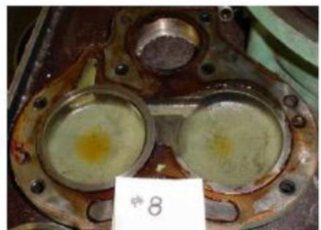
Rear Cover Varnish: 9.5 Sludge: 9.6
