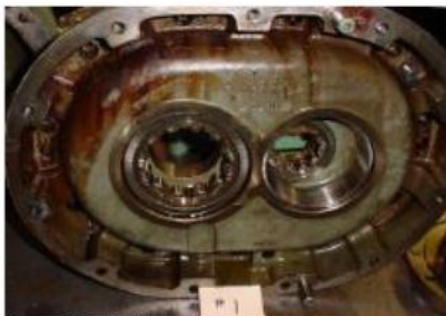
Input Shaft Housing Varnish: 6.7 Sludge: 9.6
