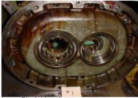
Input Shaft Housing Varnish: 6.7 Sludge: 9.6
