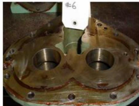
Rear cylinder plate Varnish: 9.6 Sludge: 9.6
