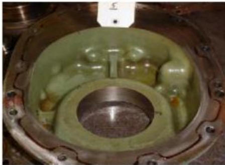
Gear Case Front Housing Varnish: 9.8 Sludge: 9.5
