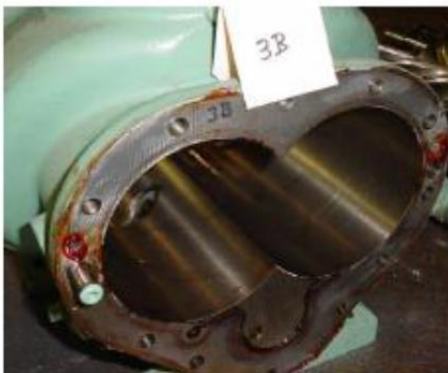
Main Rotor Housing Rear Varnish: 9.5 Sludge: 9.5
