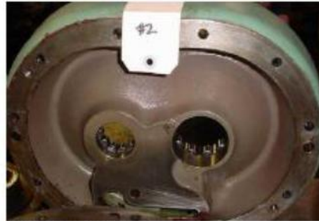
Inlet Rotor Average Varnish: 9.8 Sludge: 9.5
