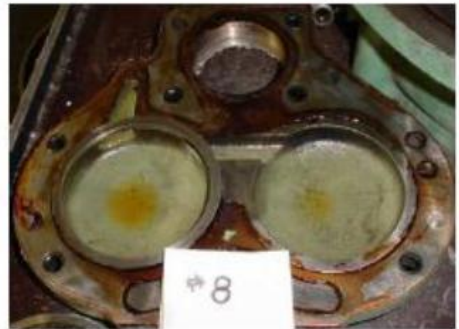
Rear Cover Varnish: 9.5 Sludge: 9.6
