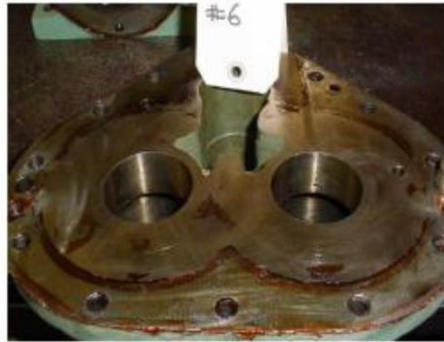
Rear cylinder plate Varnish: 9.6 Sludge: 9.6
