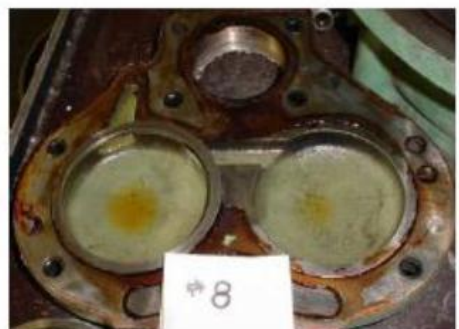
Rear Cover Varnish: 9.5 Sludge: 9.6
