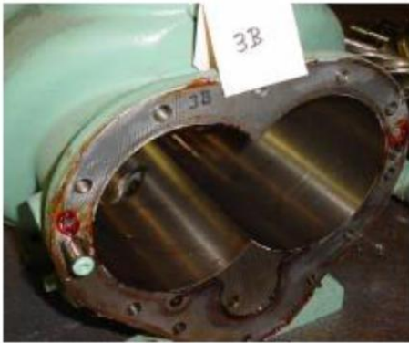
Main Rotor Housing Rear Varnish: 9.5 Sludge: 9.5
